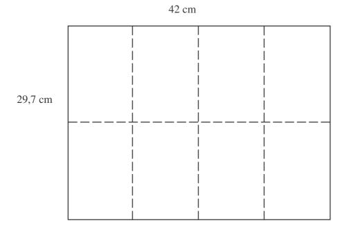
1. Divide the sheet of paper in eight parts as above, draw thin pencil lines along the divisions.
